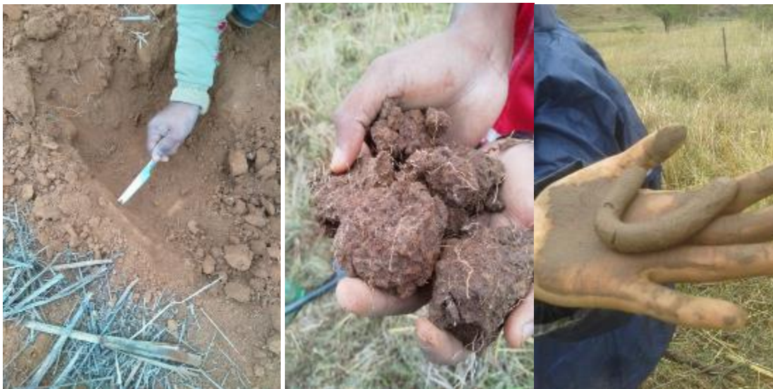
Above Left-Right: Doing the bulk density test using a knife blade. A clod of earth showing good aggregation, organic matter and fine root system. A soil sausage showing the high clay content of the soil.
