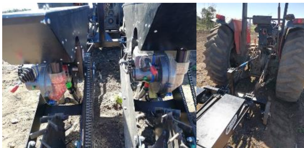
Figure 24: Right; The two-row planter with different seed types (maize, sugar beans) in the seed hoppers and Far right: a view of the planter being demonstrated in the field
