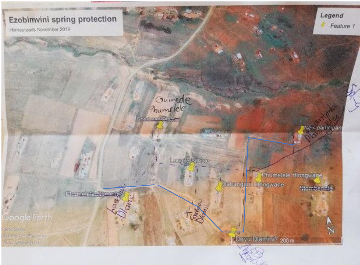
Figure 20: Creating a Google Earth map from GPS coordinates using cell phones is not very accurate, so a correction was made. The blue line indicates the main feeder pipe to participants' homesteads running along the small road to Phumelele Hlongwane's homestead.
