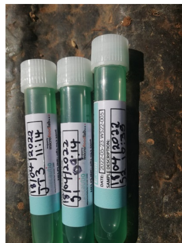
Figure 14: Right: An example of three E coli tests taken in the Stulwanae spring protection scheme in 2022/ These have turned green indicating the presence of E coli.
