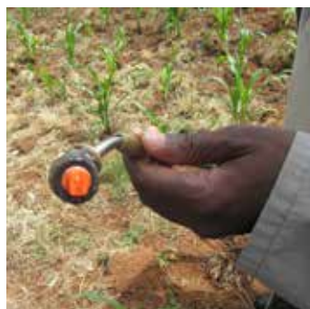
Above: The nozzles are at the tip of the sprayer where the liquid sprays out. The best nozzle for herbicides is known as an even or flat fan nozzle.
