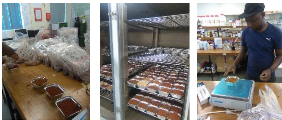
Above Left to right: Process for analysis of gravimetric soil water samples
