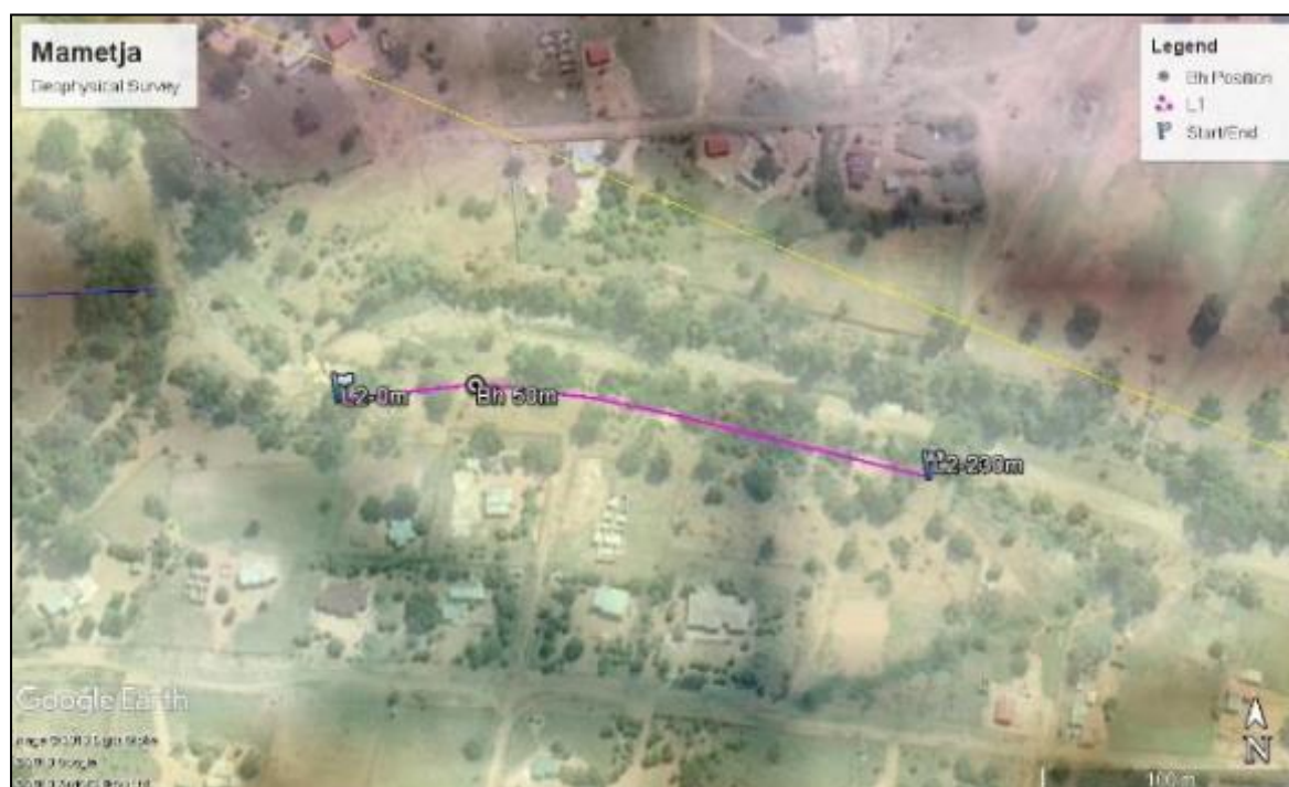
Figure 9: Assessment of Line 2 for borehole options. This line is close to the river in Sedawa and thus also has the greatest possibility of finding a strong source without deep drilling
